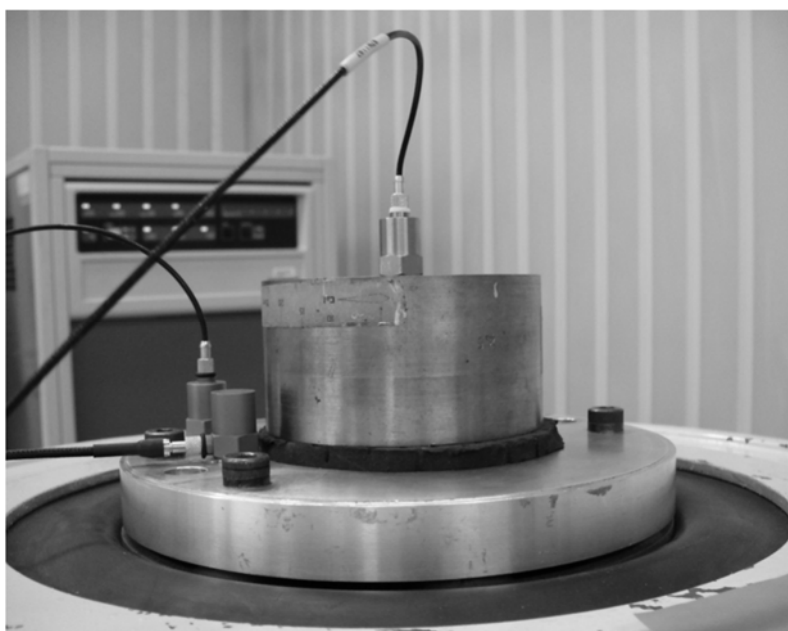
Figure 4. Sample of resilient material during measurement
