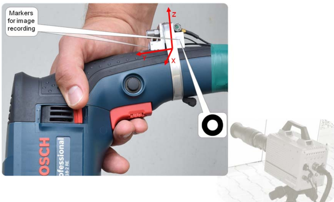
Figure 2. An example of measuring point location, orientation of the coordinate system and the transducer attachment method during high-speed camera recording
