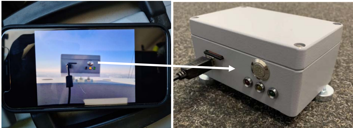
Figure 7. The Wireless transducer for vibration measurements
